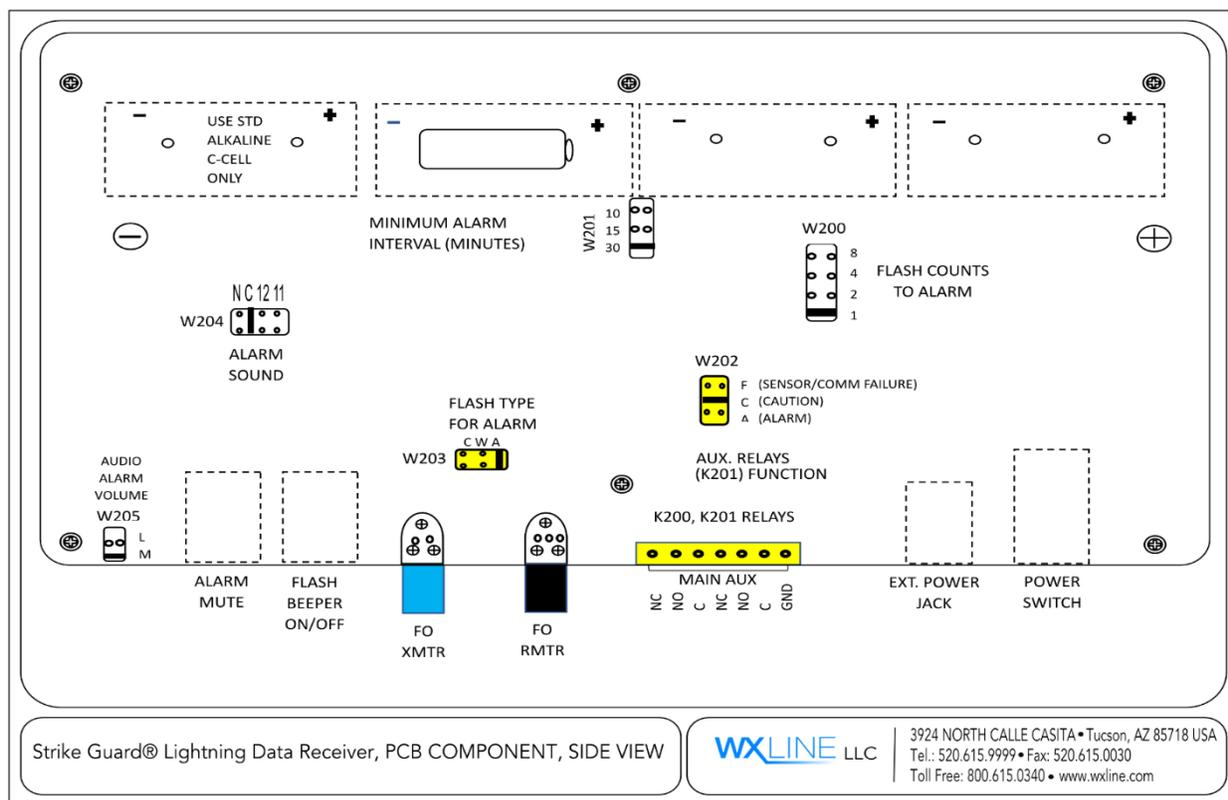
Figure 10: Lightning Data Receiver PCB Component
