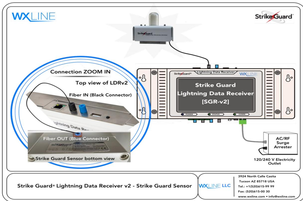
Figure 8: Strike Guard LDRv2 to Strike Guard Sensor fiber optic connection
