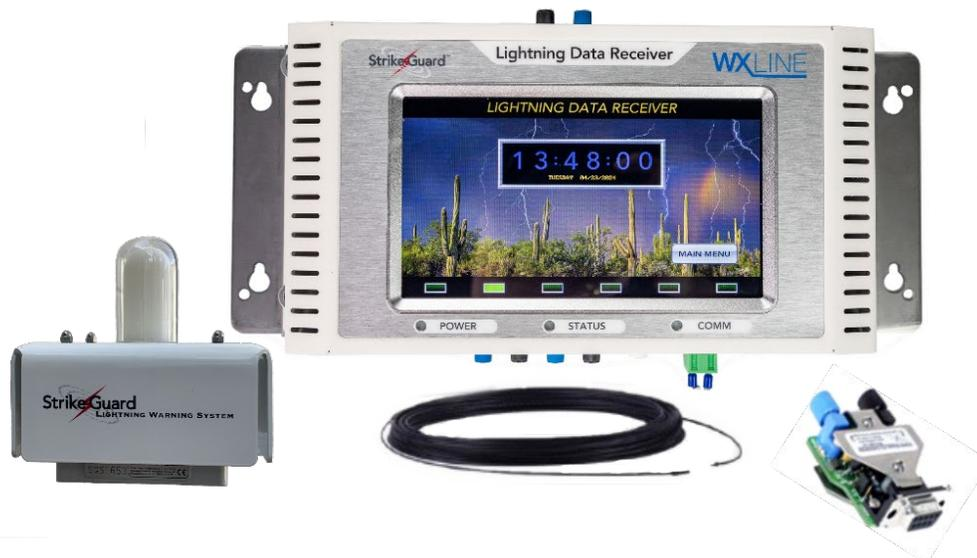
Built-in battery backup provides auxiliary power for the LDR to ensure continued operation through typical power outages. This is achieved using a pair of lead-acid batteries for the LDR-v2. The batteries are recharged automatically when primary power is restored. Primary power is 90-240 VAC, or optionally from a solar panel.
