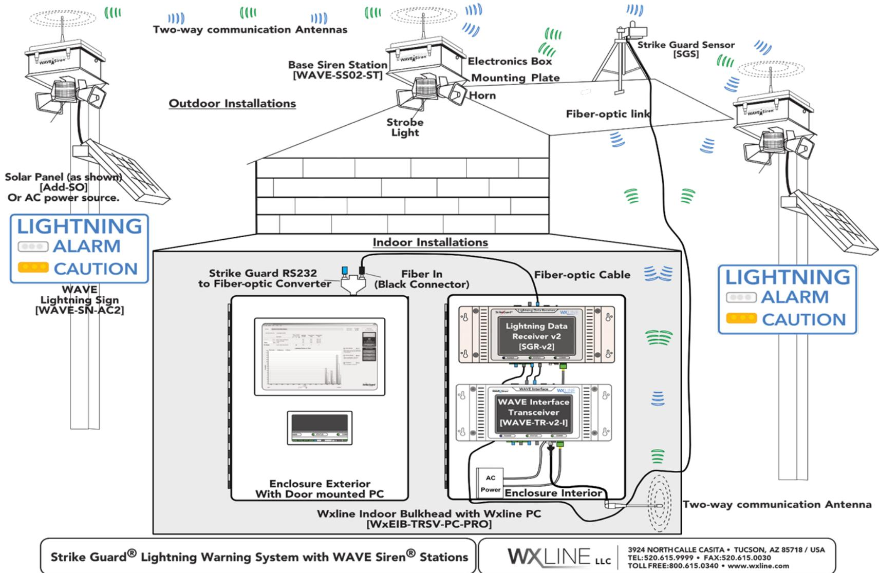
Figure 14: Strike Guard Lightning Warning System with WAVE Siren Stations
