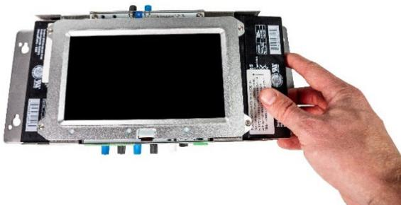
Replace the two 6v lead-acid batteries in the Lightning Data Receiver Standard edition every 1 to 2 years even if the Low Battery indication is not showing to prevent battery leakage from damaging the circuit board. Replace the lead-acid batteries only with the same type and carefully check to ensure that battery polarity is correct on all cells. Never allow fingers to touch the
