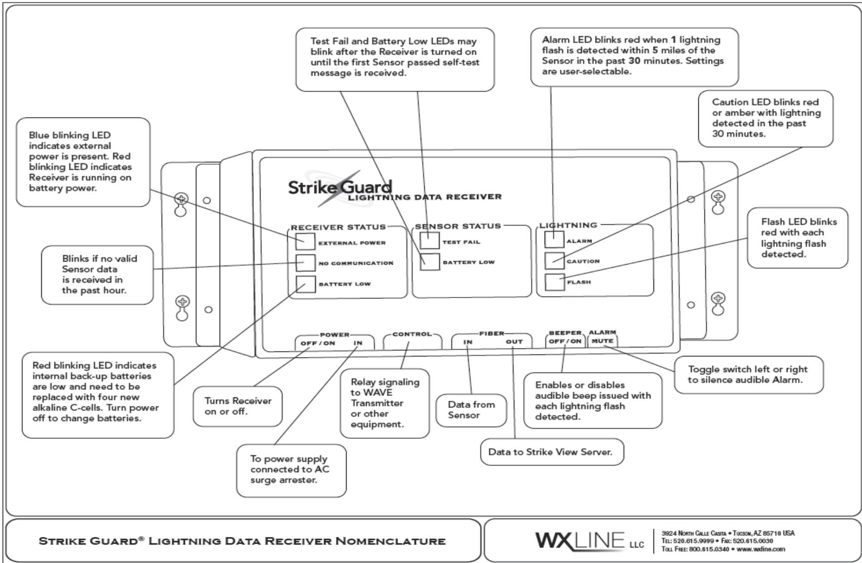
Figure 12: Lightning Data Receiver Nomenclature
