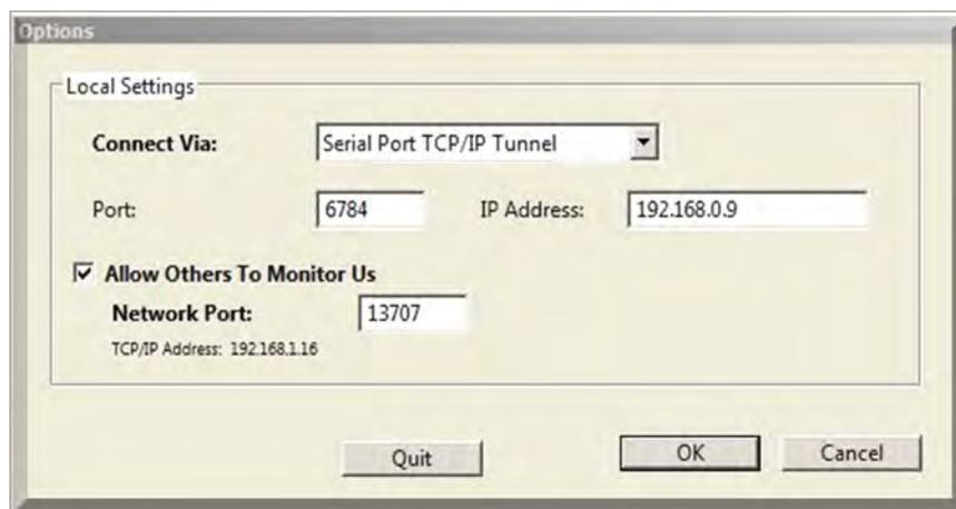
Figure 2: A Strike View Server Network Settings Window using a TCP/Tunnel to monitor a remote Strike Guard Sensor with NL201 Serial/LAN Interface.
