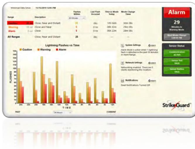
Strike View Server enables the user to connect a computer to a Strike Guard Lightning Data Receiver, monitor incoming data, and share data across a LAN.
