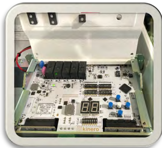
Figure 9: DIP switches under front cover of Siren Station
