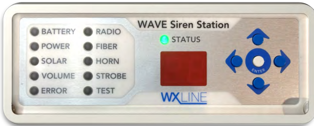
Figure 8: Interface panel and diagnostic digital read-out
