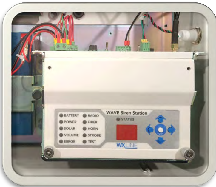
Figure 6: WAVE Siren electronics cage
